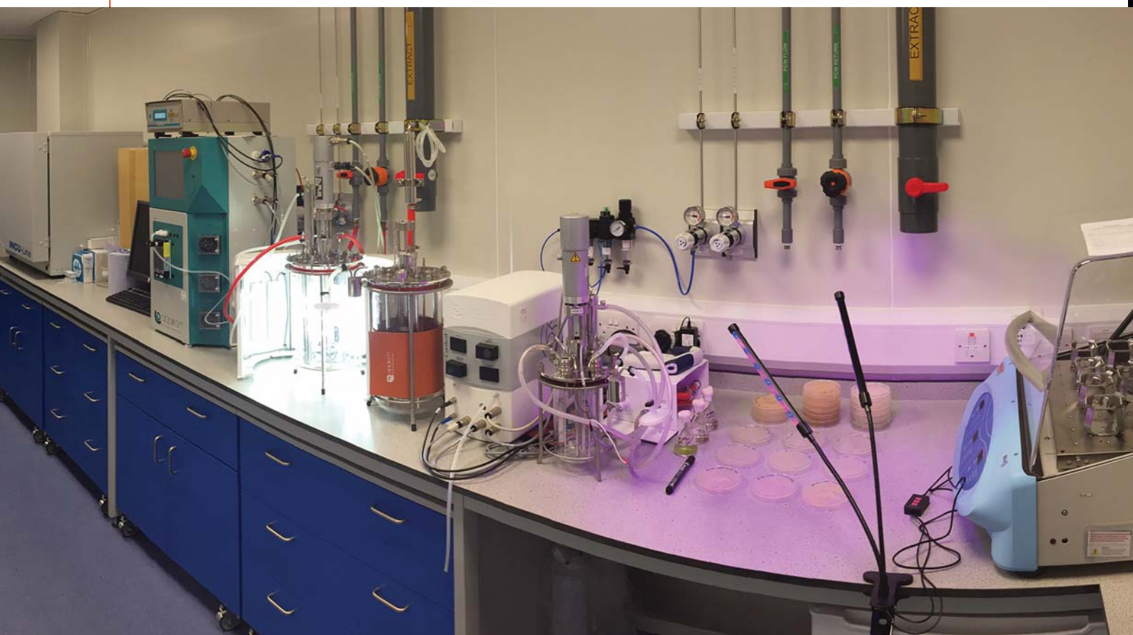
FlexBio's microbial fermentation lab – Allows media optimisation of cells in plate, flask and fermenter up to 5 litre scale
